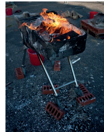
Left: Paper kiln in which clay items are surrounded with wood encased in layers of clay-soaked paper
