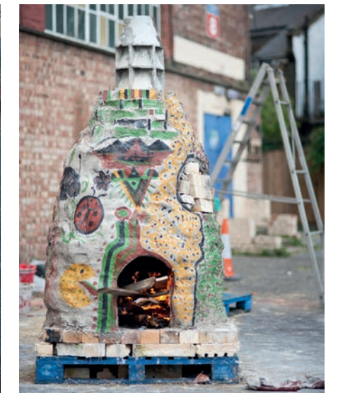
Left: Paper kiln in which clay items are surrounded with wood encased in layers of clay-soaked paper
