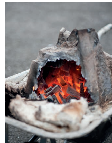
Left: Paper kiln in which clay items are surrounded with wood encased in layers of clay-soaked paper
